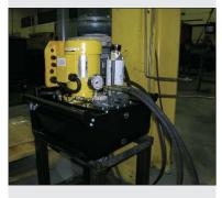
Z-class pump model number **ZW5020HK-FHT01** is used to provide pressure and flow to six machining fixtures.
